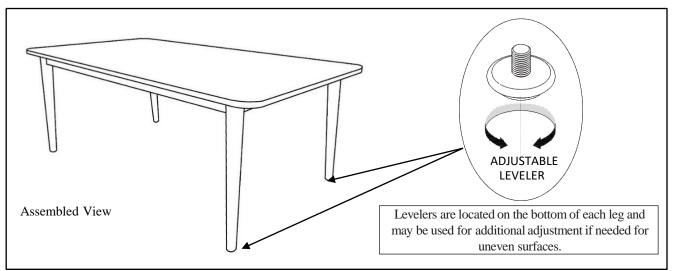
Assembly is now complete and the product is ready for use. Adjustable levelers are located on the bottom of each leg and may be adjusted by turning outwards, counter-clockwise to help account for uneven surfaces. NOTE: Hardware may loosen over time. Periodically check that all connections remain tight and adjust as needed.
