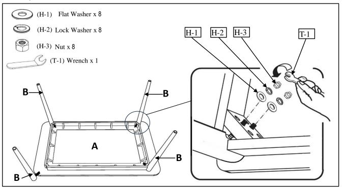
Place the Tabletop (A) upside down onto a padded, non-marring surface. Position the Legs (B) at each corner of the Tabletop (A) by inserting the hanger bolts through the holes. Secure by engaging Flat Washers (H-1), Lock Washers (H-2) and Nuts (H-3), stacking the hardware in the order as shown. Once engaged, fully tighten using the provided Wrench (T-1). DO NOT OVERTIGHTEN. Repeat for all Legs (B).
